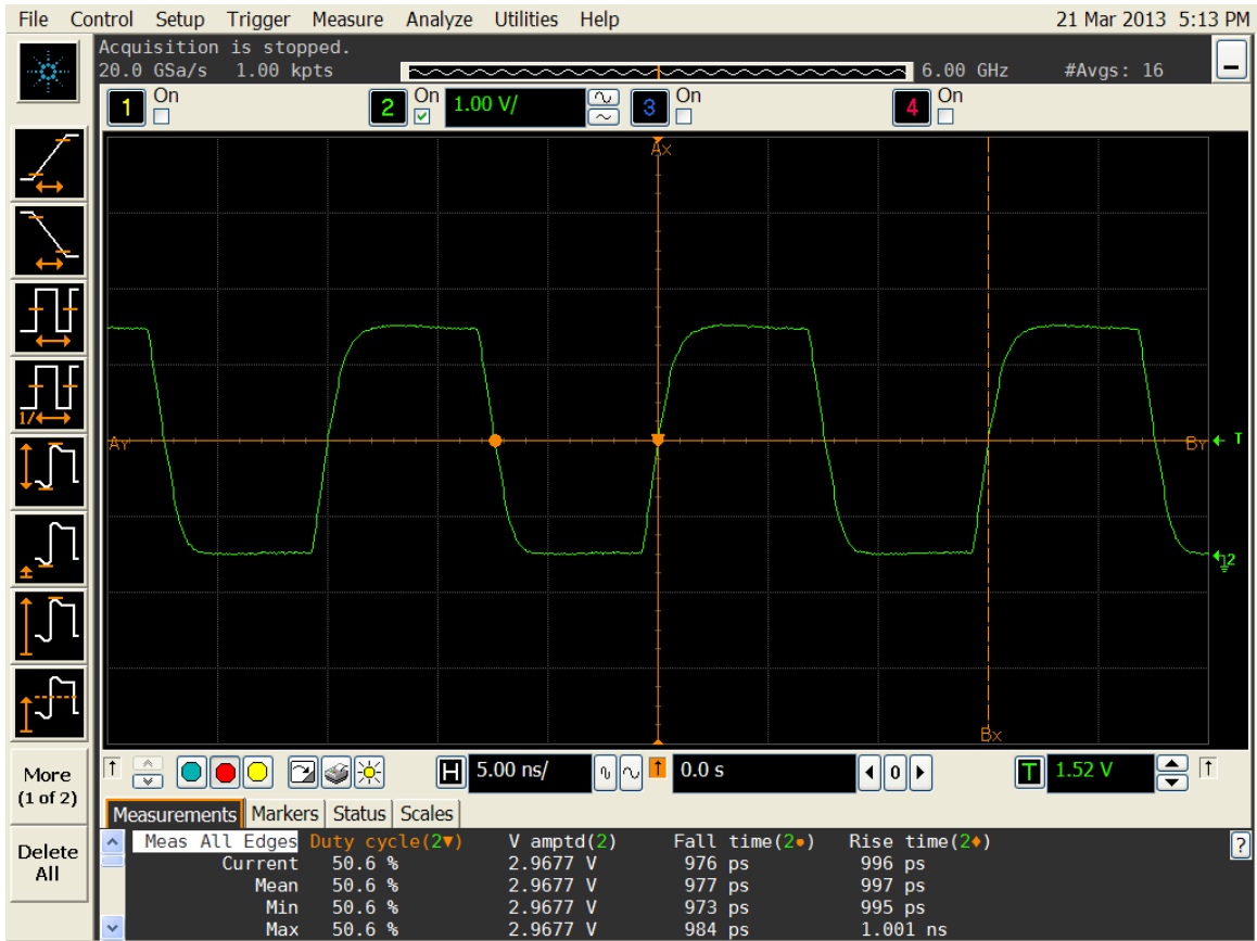
Figure 4. Duty cycle, Rise/Fall time and Amplitude 3.0V
