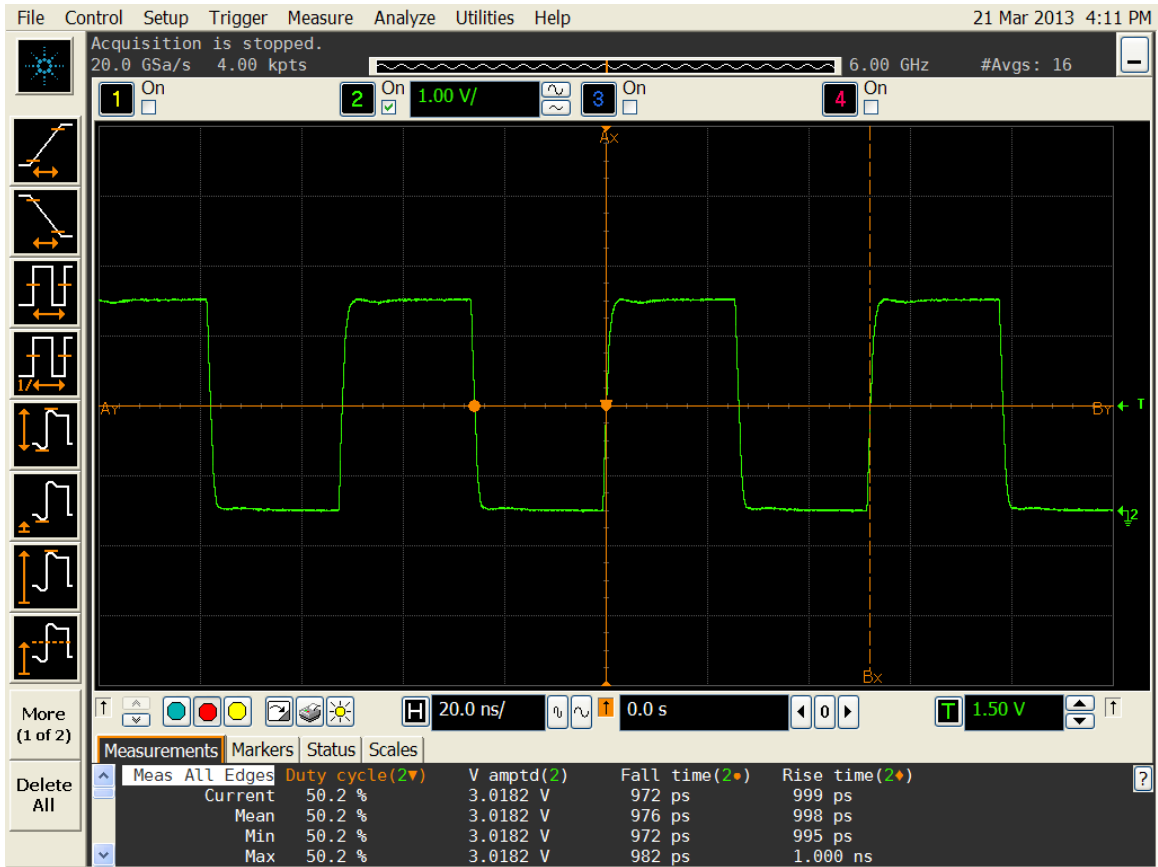
Figure 4. Duty cycle, Rise/Fall time and Amplitude 3.0V
