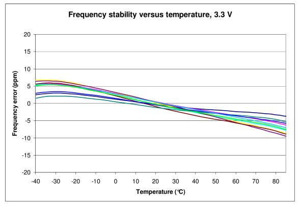
Figure 10. Frequency stability versus temperature, 3.3 V
