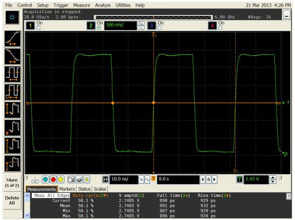
Figure 3. Duty cycle, Rise/Fall time and Amplitude 2.8V
