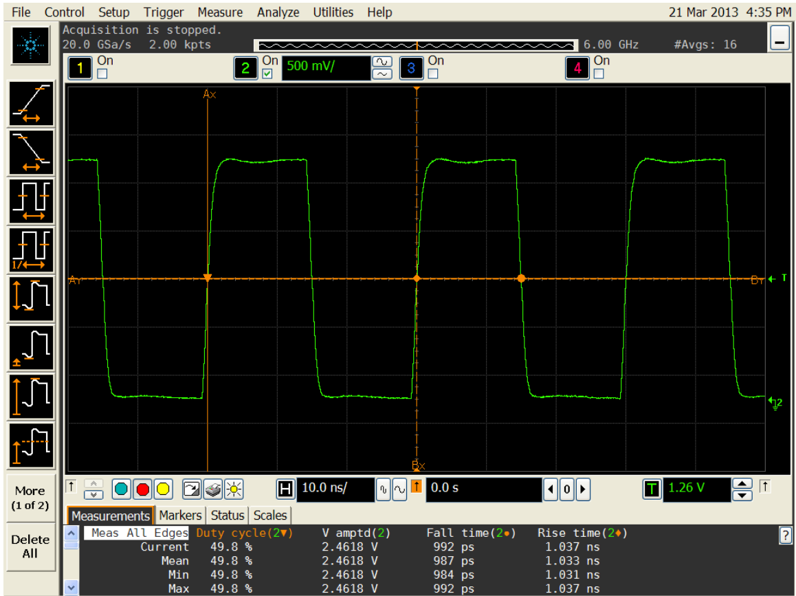
Figure 2. Duty cycle, Rise/Fall time and Amplitude 2.5V
