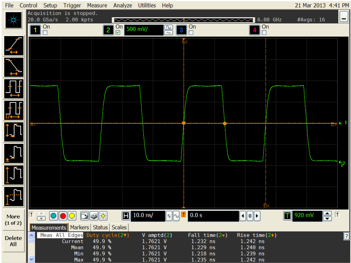
Figure 1. Duty cycle, Rise/Fall time and Amplitude 1.8V
