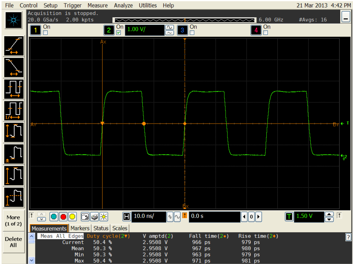
Figure 4. Duty cycle, Rise/Fall time and Amplitude 3.0V
