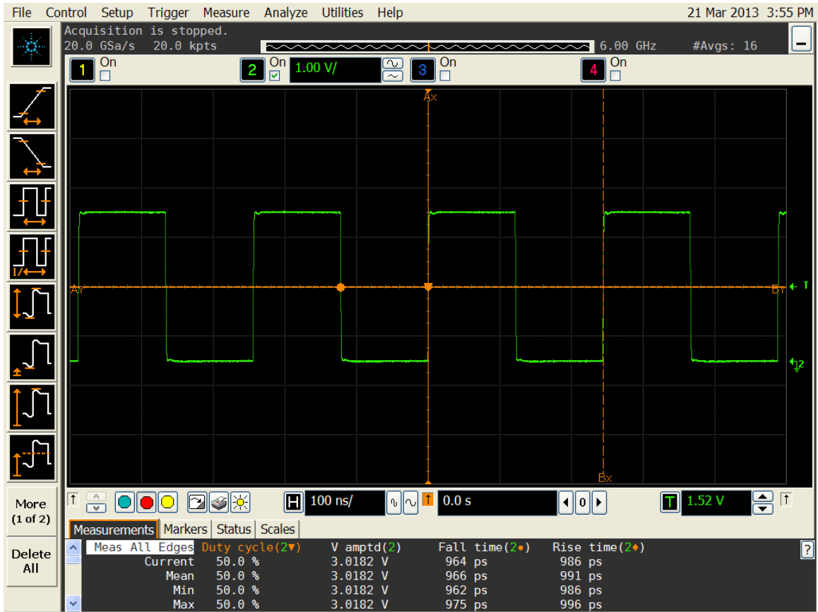
Figure 4. Duty cycle, Rise/Fall time and Amplitude 3.0V
