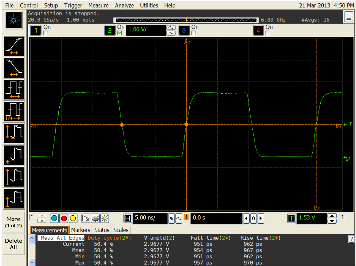
Figure 4. Duty cycle, Rise/Fall time and Amplitude 3.0V
