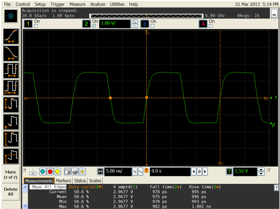
Figure 4. Duty cycle, Rise/Fall time and Amplitude 3.0V
