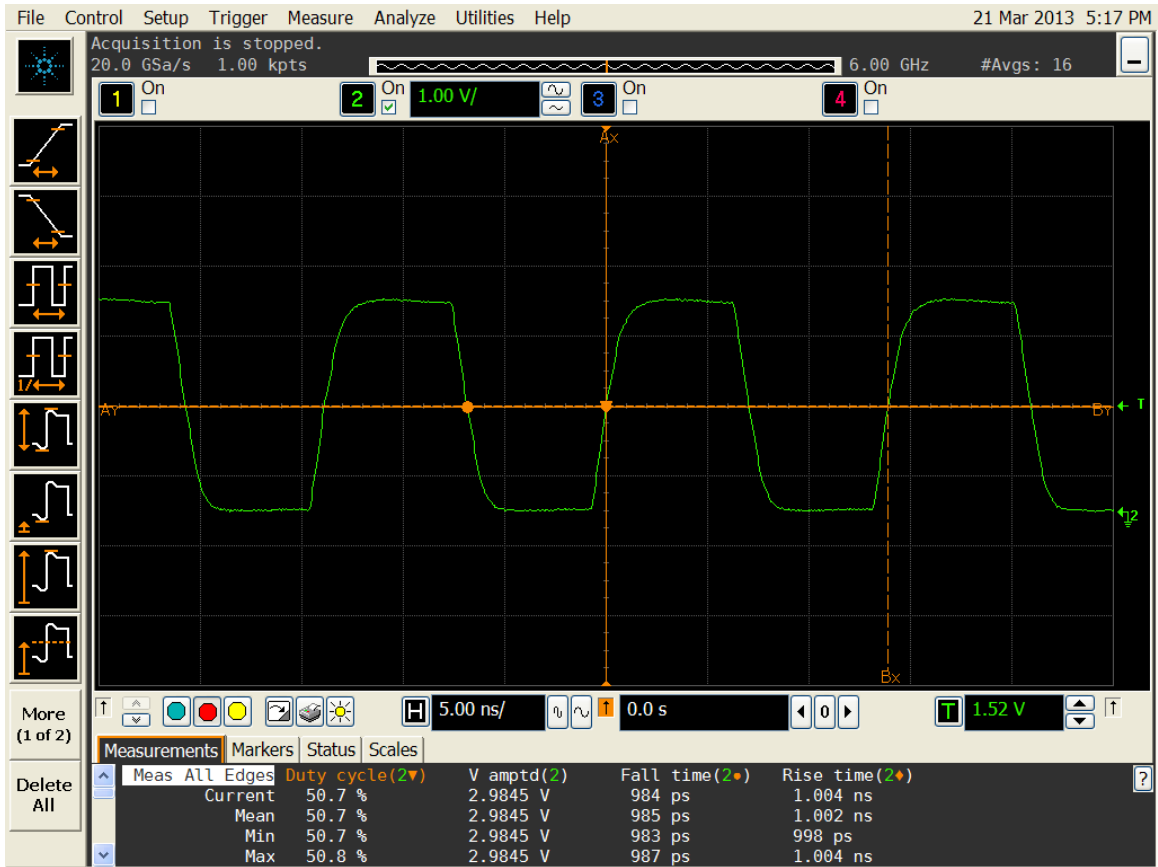
Figure 4. Duty cycle, Rise/Fall time and Amplitude 3.0V
