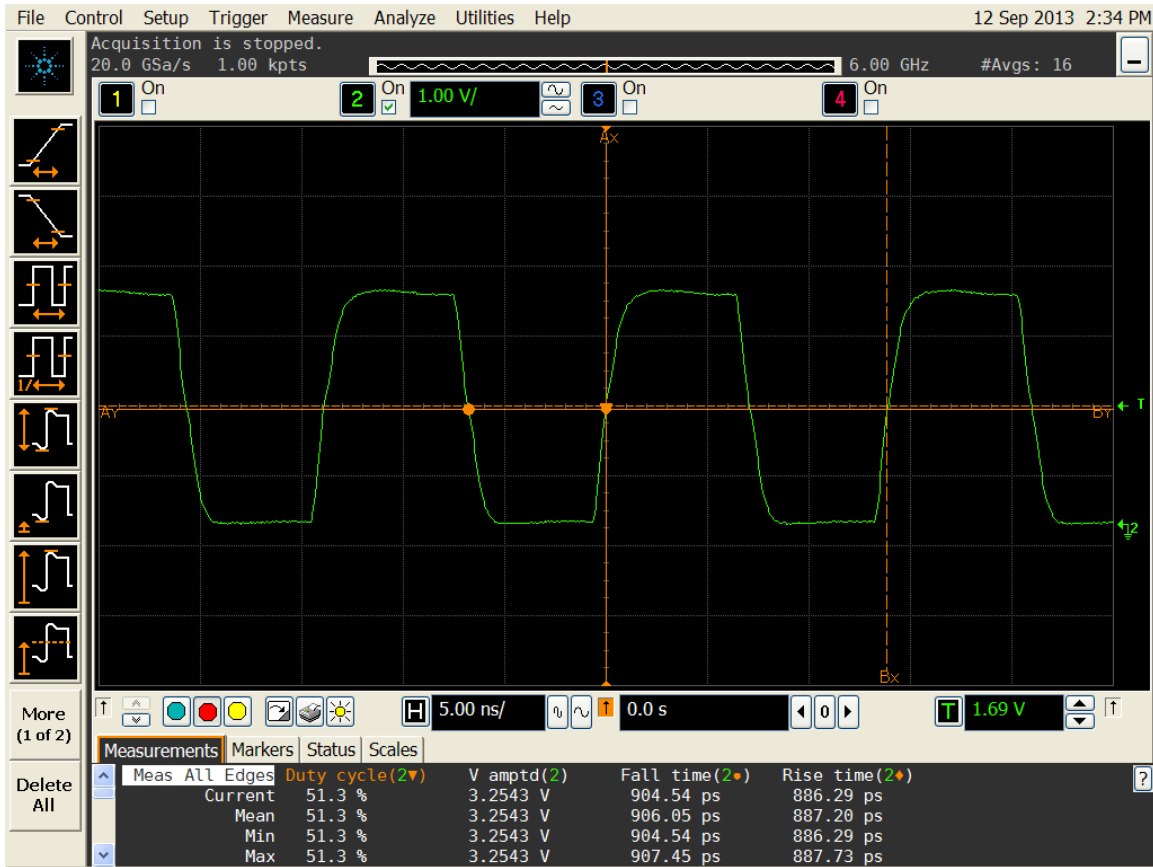
Figure 5. Duty cycle, Rise/Fall time and Amplitude 3.3V
