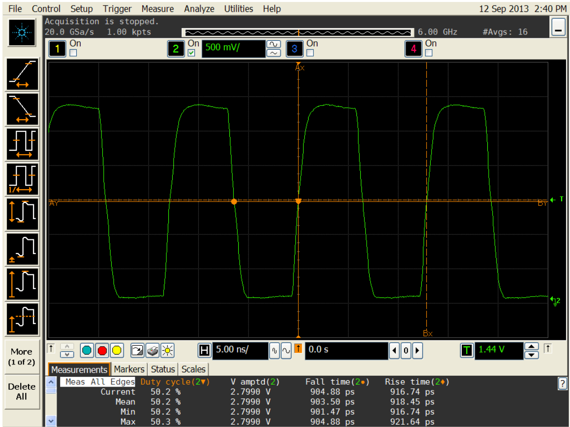
Figure 3. Duty cycle, Rise/Fall time and Amplitude 2.8V
