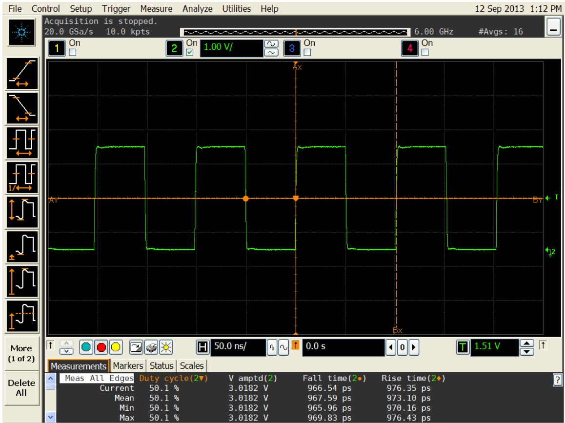
Figure 4. Duty cycle, Rise/Fall time and Amplitude 3.0V
