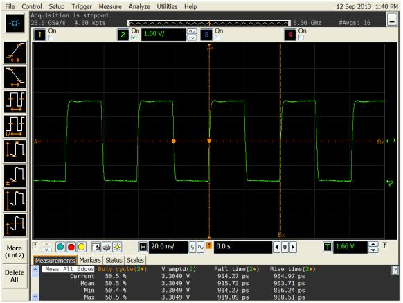
Figure 5. Duty cycle, Rise/Fall time and Amplitude 3.3V
