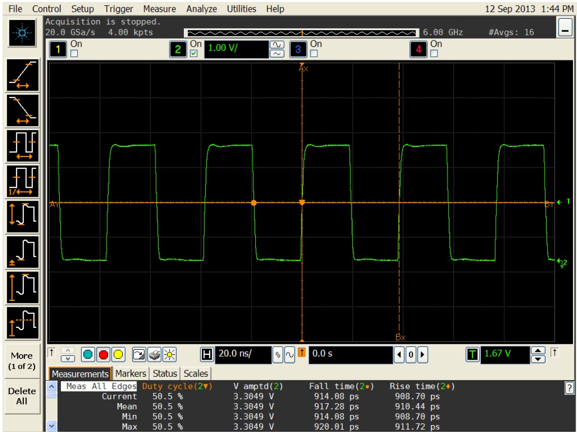
Figure 5. Duty cycle, Rise/Fall time and Amplitude 3.3V
