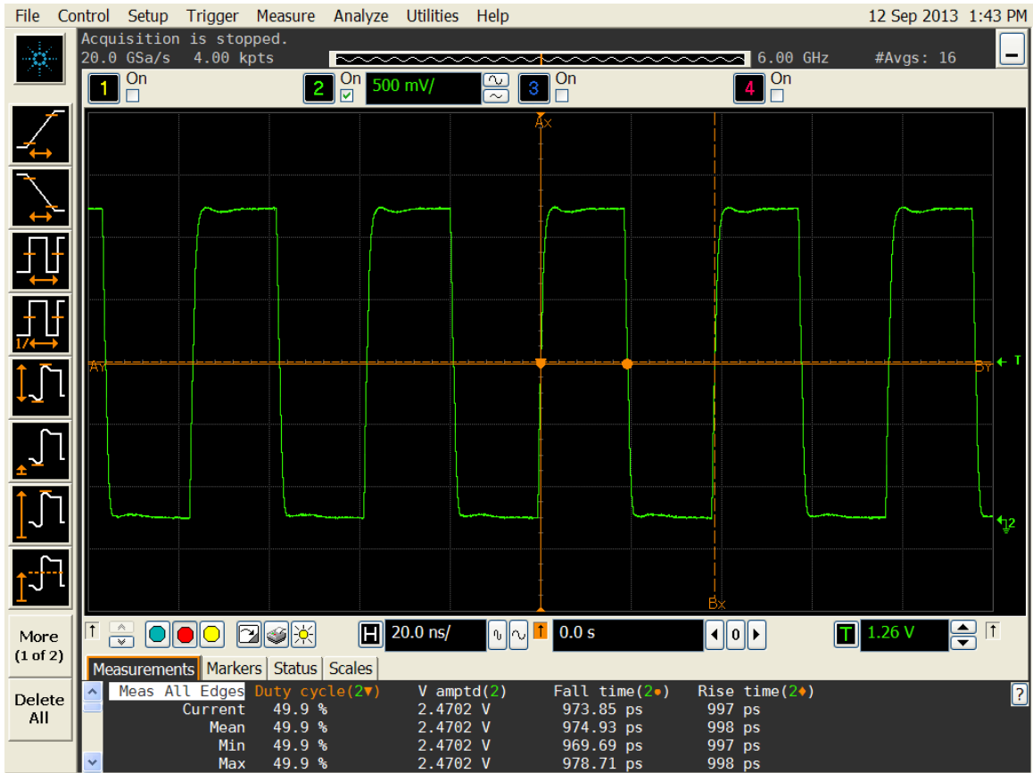
Figure 2. Duty cycle, Rise/Fall time and Amplitude 2.5V
