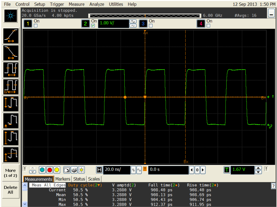
Figure 5. Duty cycle, Rise/Fall time and Amplitude 3.3V
