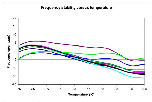
Figure 6. Frequency stability\* versus temperature
