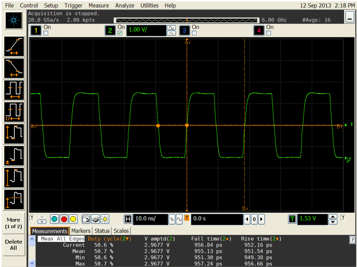
Figure 4. Duty cycle, Rise/Fall time and Amplitude 3.0V
