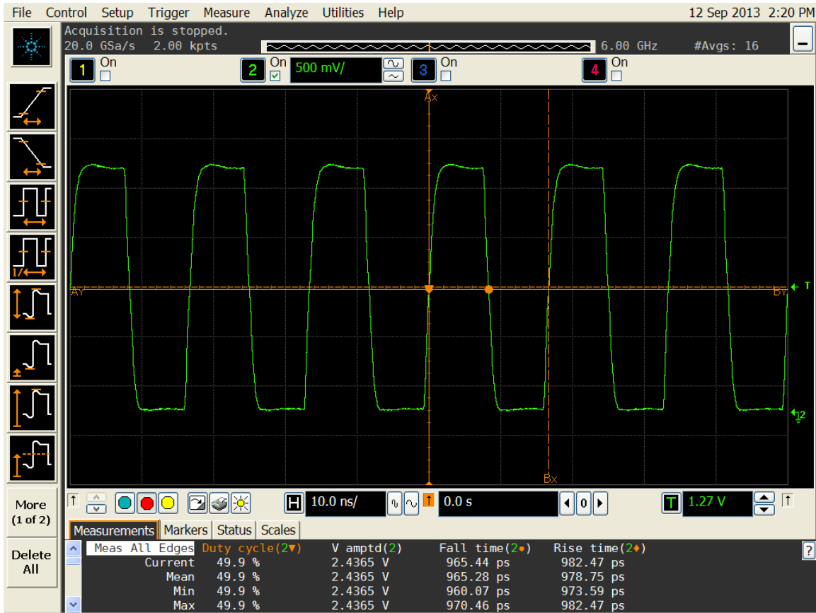
Figure 2. Duty cycle, Rise/Fall time and Amplitude 2.5V
