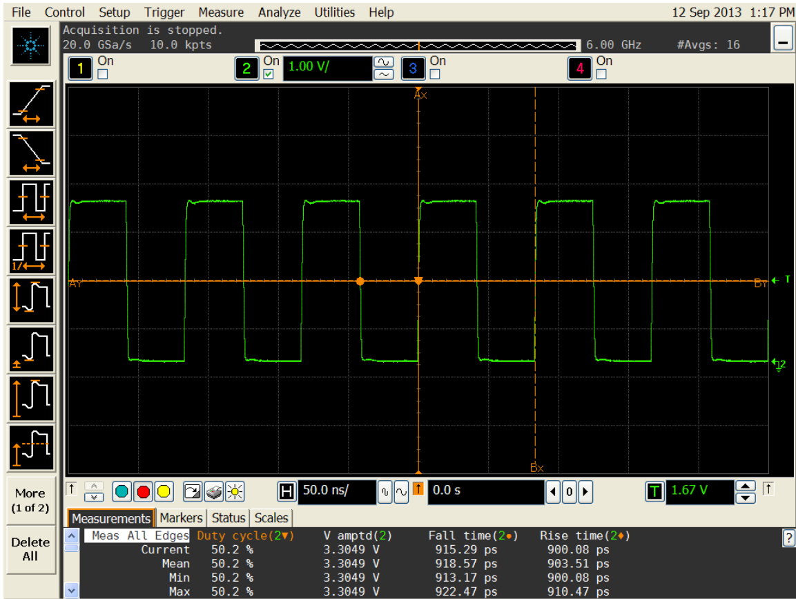
Figure 5. Duty cycle, Rise/Fall time and Amplitude 3.3V
