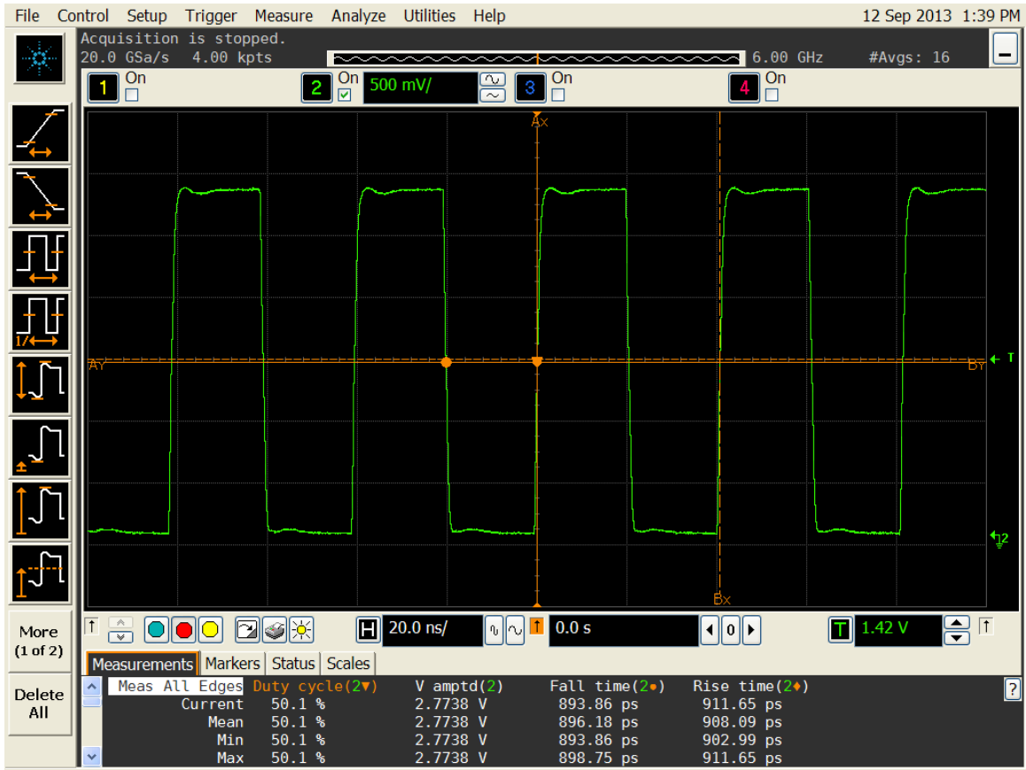
Figure 3. Duty cycle, Rise/Fall time and Amplitude 2.8V
