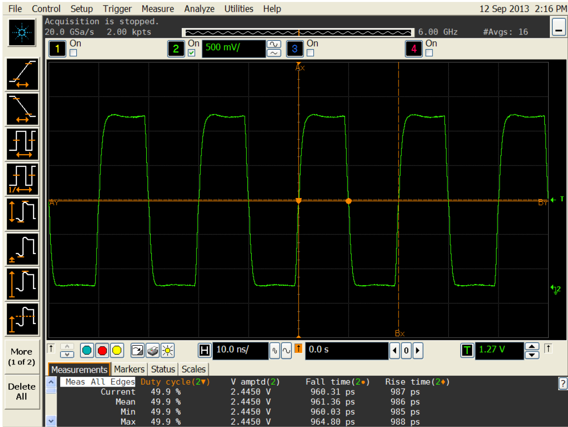
Figure 2. Duty cycle, Rise/Fall time and Amplitude 2.5V
