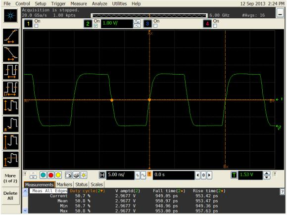
Figure 4. Duty cycle, Rise/Fall time and Amplitude 3.0V
