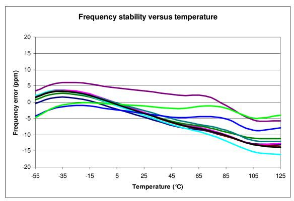
Figure 6. Frequency stability\* versus temperature
