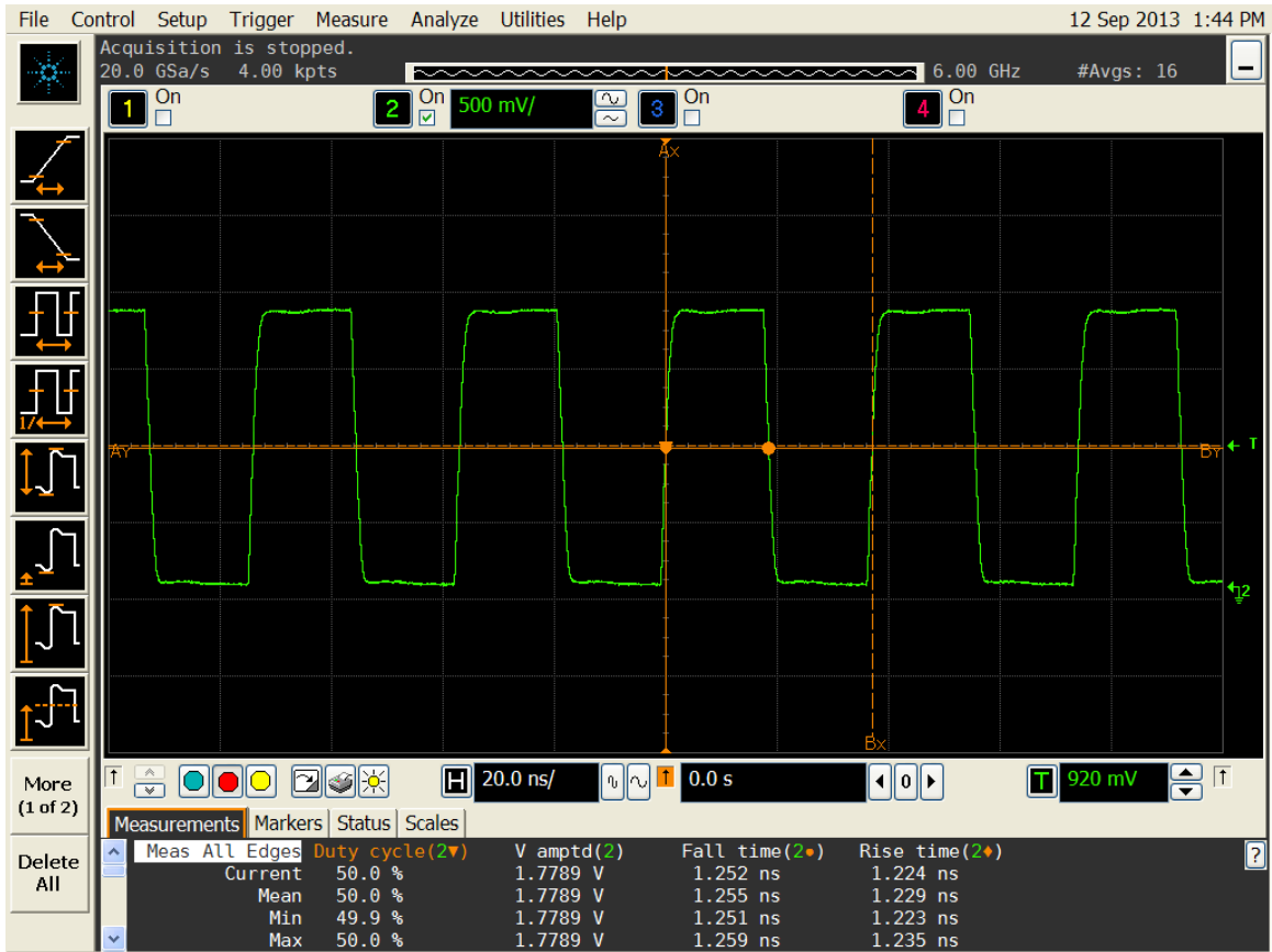
Figure 1. Duty cycle, Rise/Fall time and Amplitude 1.8V
