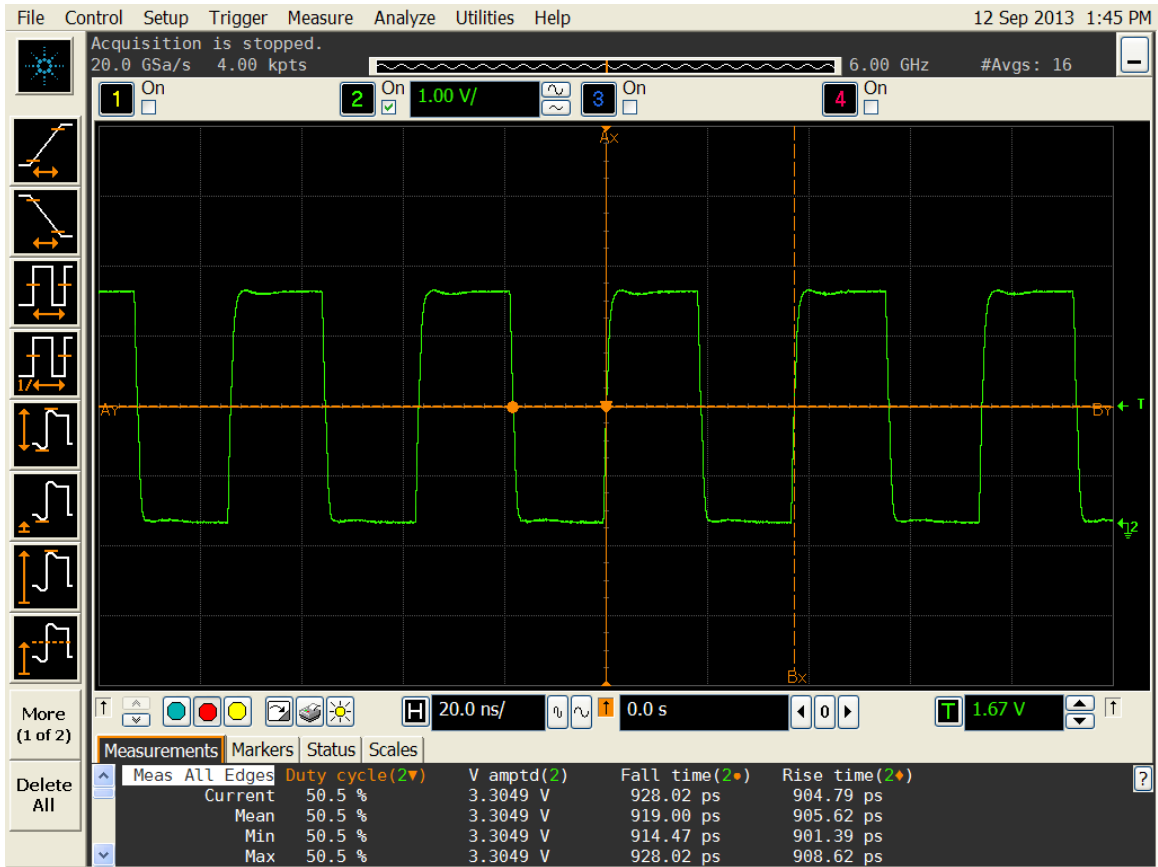
Figure 5. Duty cycle, Rise/Fall time and Amplitude 3.3V
