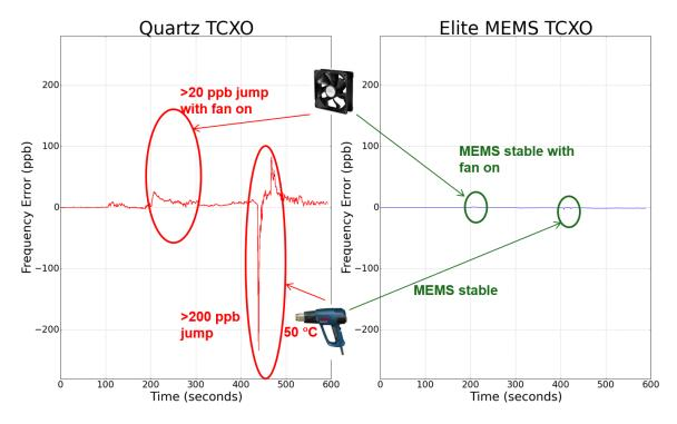
Figure 2. Quartz TCXOs are sensitive to heat, airflow, and rapid temperature shifts, exhibiting significant frequency variations, while MEMS TCXOs are extremely stable under these conditions.
